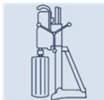
Electric wet core drill with diamond core bit (HILTI D150 or DD250 recommended) and core drill stand (« tower »)
